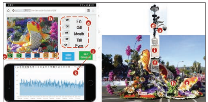
FIGURE 4. Interaction between the audiences and the Singpoli parade float; (a)→(b): the path from a camera to a viewing screen; (c) → (d): the camera control path; (e) → (f) → (g): the fish gesture control path; (h) → (i) → (j): the sensor data display path; clicking (j) to shown the time series chart in (k)
