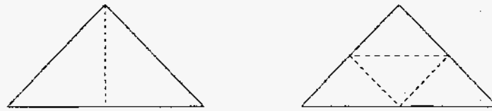
FIG. 3. On the left, a triangle divided with bisection; on the right, a triangle divided by using regular refinement
