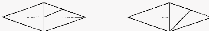
FIG. 2. On the left, a conforming mesh; on the right, a nonconforming mesh
