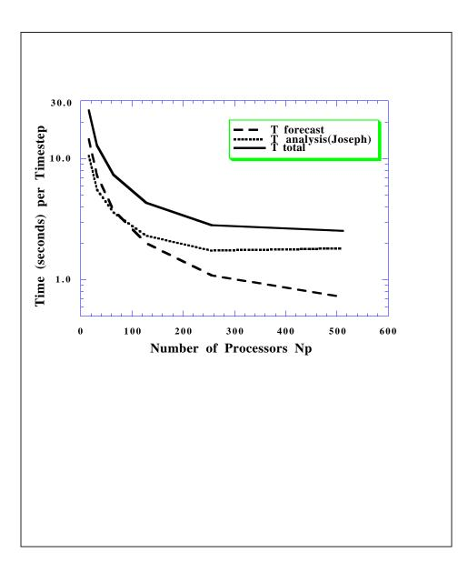
Figure 5. The actual time (seconds) per timestep of the forecast step, the analysis step, and the full Kalman filter on the Intel Paragon for medium resolution  $(4^{\circ} \times 5^{\circ})$  using Covariance Decomposition and the Joseph form Eq. (13).
