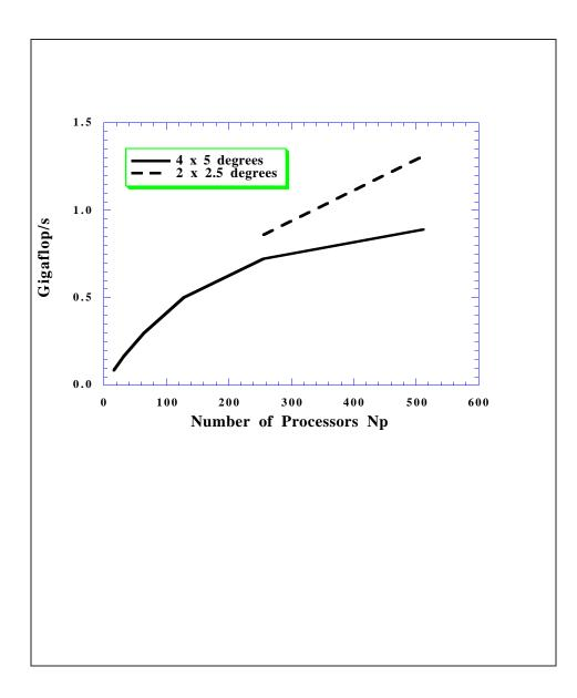
Figure 7. Gigaflop/s rates for the full Kalman filter at medium and high resolution on the Intel Paragon. These numbers were obtained for the optimal form of the analysis step, Eq. (14).
