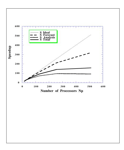
Figure 3. The actual speedups for the forecast step, the analysis step, and the full Kalman filter on the Intel Paragon for medium resolution  $(4^{\circ} \times 5^{\circ})$  using Covariance Decomposition and the Joseph form Eq. (13).
