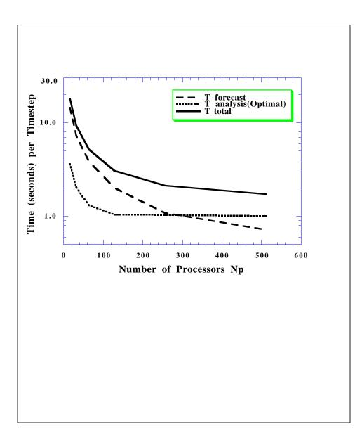
Figure 6. The actual time (seconds) per timestep of the forecast step, the analysis step, and the full Kalman filter on the Intel Paragon for medium resolution  $(4^{\circ} \times 5^{\circ})$  using Covariance Decomposition and the optimal form Eq. (14).
