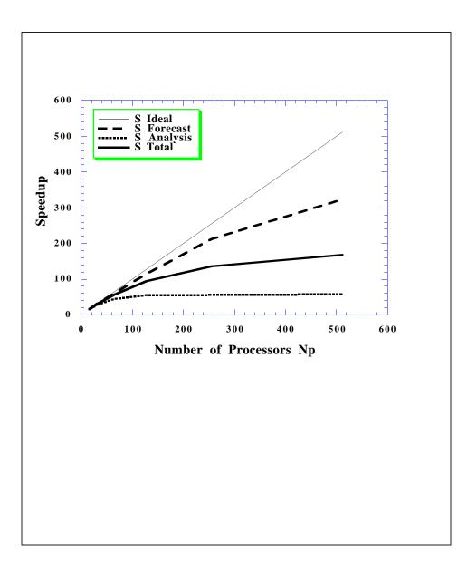
Figure 4. The actual speedups for the forecast step, the analysis step, and the full Kalman filter on the Intel Paragon for medium resolution  $(4^{\circ} \times 5^{\circ})$  using Covariance Decomposition and the optimal form Eq. (14).
