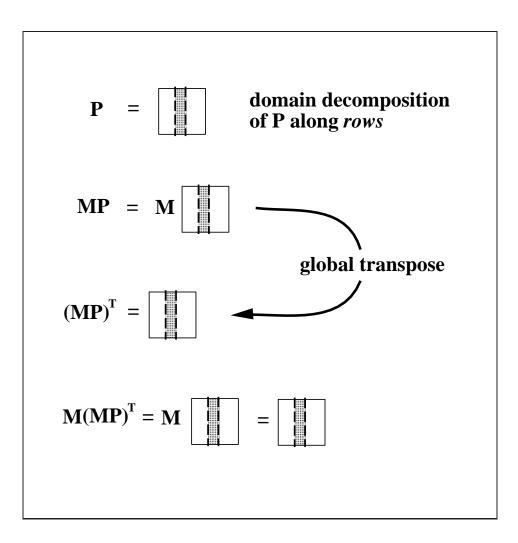
Figure 1 (b). Schematic for the *Covariance Decomposition* approach for storing large size- $n^2$  matrices and performing  $M(MP)^T$ .
