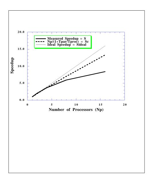
Figure 2. Speedup curves for the domain decomposed van Leer transport algorithm implemented on the Intel Delta.
