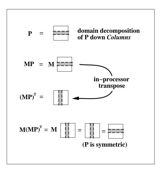
Figure 1 (a). Schematic for the *Operator Decomposition* approach for storing large size- $n^2$  matrices and performing  $M(MP)^T$ .
