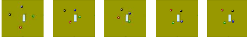
Fig. 6 Four agents (rendered as circular discs), traveling in opposite directions form a vortex as they maneuver around an obstacle.
