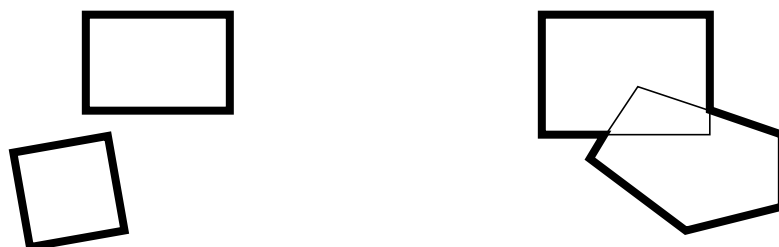
Figure 5-5. Examples of unions of two convex sections resulting in a non-convex section
