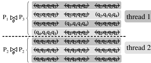
Figure 17: Allocating search spaces using round-robin outer allocation for building P_4 to two threads.
