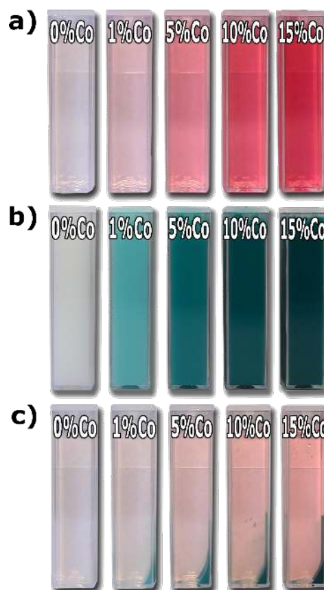
Figure 5: (a) Photographs of the \text{Zn}_{1-x}\text{Co}_x\text{O} precursor in ethylene glycol where the color varies with the composition. (b) Photographs of nanoparticle dispersions in ethylene glycol after microwave solvothermal synthesis. (c) Photographs of nanoparticle dispersions in ethylene glycol after sedimentation.
