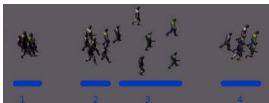
Figure 9: Sketch-based simulation. RVO2 agents are made to travel grouped, then disperse and then regroup again. Four consecutive states are shown.
