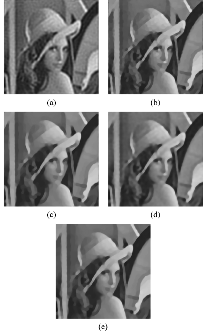
Fig. 4. Restorations of the Lena image blurred with a Gaussian PSF with variance 9 and 20-dB BSNR using the (a) MOL method (ISNR = 2.45 dB), (b) BFO1 method (ISNR = 3.02 dB), (c) BFO2 method (ISNR = 2.47 dB), (d) ALG1 method (ISNR = 3.06 dB), and (e) ALG2 method (ISNR = 2.58 dB).
