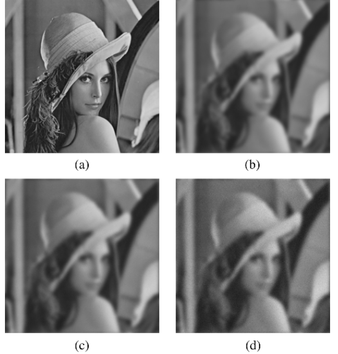
Fig. 2. (a) Lena image; degraded with a Gaussian shaped PSF with variance 9 and Gaussian noise of variance: (b) 0.16 (BSNR = 40 dB), (c) 1.6 (BSNR = 30 dB), (d) 1 (BSNR = 20 dB).
