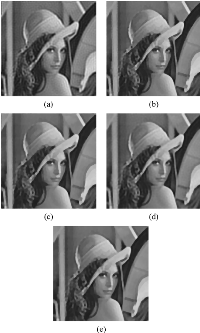
Fig. 3. Restorations of the Lena image blurred with a Gaussian PSF with variance 9 and 40-dB BSNR using the (a) MOL method (ISNR = 3.90 dB), (b) BFO1 method (ISNR = 4.72 dB), (c) BFO2 method (ISNR = 4.5 dB), (d) ALG1 method (ISNR = 4.84 dB), and (e) ALG2 method (ISNR = 4.64 dB).
