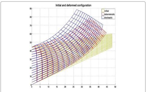
**Fig. 5** Cook's membrane—large strain elasto-plasticity, undeformed grid [initial], deformations with mean properties [deterministic], and mean of the deformation with stochastic properties [stochastic], from [18,24,25]
