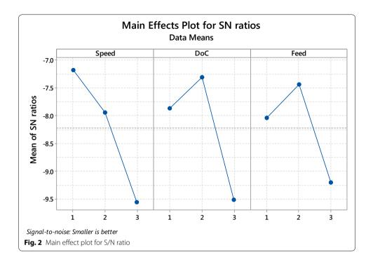
From Figs. 1 and 2 the lines connecting level of factors are not horizontal indicating each factor affects differently. The minimum value of the mean and the maximum value of S/N ratio is observed at level 1 (200 rpm) of speed, level 2 (1.2 mm) depth of cut and level 2 (40 mm/min) feed. These levels of control factor present optimal setting for minimization of surface roughness.
