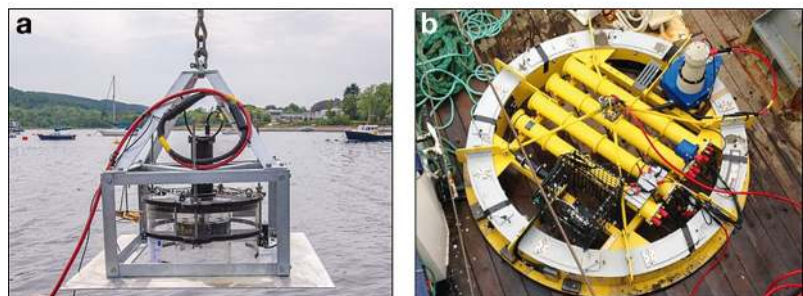
Fig. 2. Benthic flumes used in the study. (a) Voyager I mini-flume; (b) plan view of the Voyager II benthic flume
