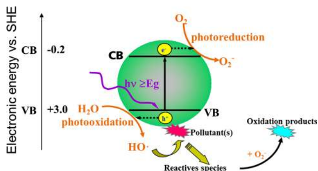
Fig. 1 Schematic representation of the photocatalytic mechanism (redrawn from Ref 2, 6)
