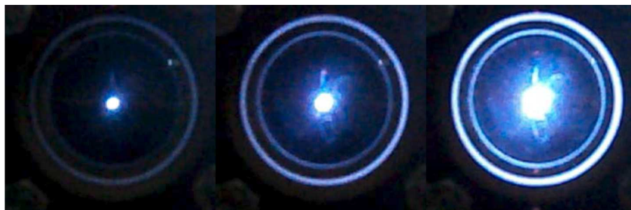
Fig. 2. Photos of a nanosecond overvoltage discharge between the copper electrodes at pulse repetition frequencies of 40, 150, and 1000 Hz (from left to right)
