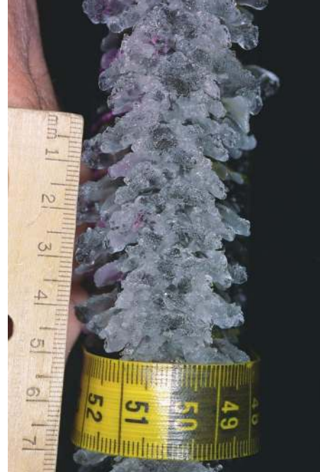
Figure 46. Complete scallop at \Lambda=40^\circ , V=150 mph, T=25^\circ\text{F} , \text{LWC}=0.75\text{g/m}^3 , \text{MVD}=20\mu\text{m} , \tau=5\text{min} . Direction of flow is from bottom to top, scale of ruler is in centimeters, smallest division 1 millimeter.
