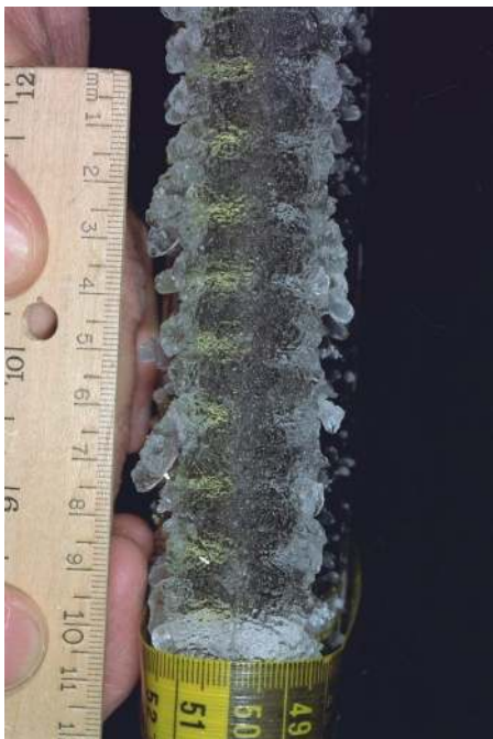
Figure 34. Front view of ice accretion showing the ice of the attachment line zone covering most of the feathers in the glaze ice feathers zone. \Lambda=15^\circ , V=100 mph, T=25^\circ\text{F} , \text{LWC}=0.75\text{g}/\text{m}^3 , \text{MVD}=20\mu\text{m} , \tau=10\text{min} . Direction of flow is from bottom to top, scale of ruler is in centimeters, smallest division 1 millimeter.
