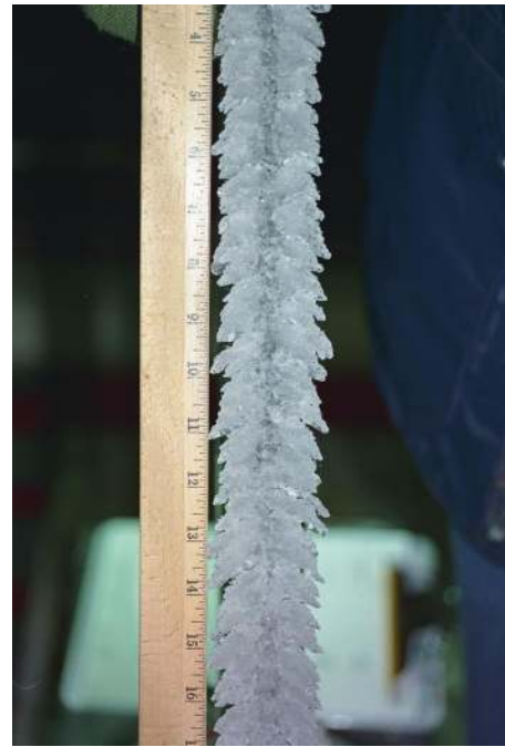
Figure 9. Front view of ice accretion. Run conducted with 1996 spray system. \Lambda=30^\circ , V=200 mph, T=25^\circ\text{F} , \text{LWC}=0.75\text{g/m}^3 , \text{MVD}=20\mu\text{m} , \tau=10\text{min} . Direction of flow is from bottom to top, scale of ruler is in inches.
