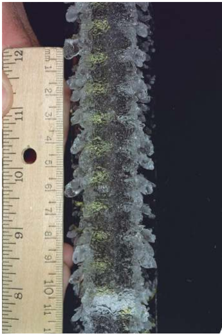
Figure 36. Front view of ice accretion showing the formation of scallop tips. \Lambda=25^\circ , V=100 mph, T=25^\circ\text{F} , \text{LWC}=0.75\text{g/m}^3 , \text{MVD}=20\mu\text{m} , \tau=10\text{min} . Direction of flow is from bottom to top, scale of ruler is in centimeters, smallest division 1 millimeter.
