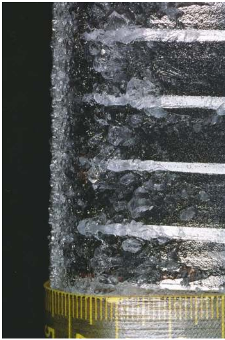
Figure 28. Side view of ice accretion showing individual feathers in the glaze ice feathers zone. \Lambda=0^\circ , V=100 mph, T=25^\circ\text{F} , \text{LWC}=0.75\text{g/m}^3 , \text{MVD}=20\mu\text{m} , \tau=5\text{min} . Scale of ruler is in centimeters, smallest division 1 millimeter.
