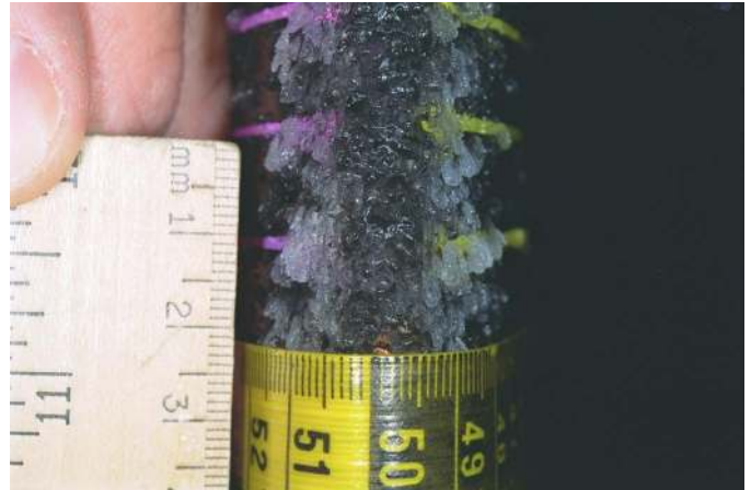
Figure 17. Front view of the ice accretion showing the top part of large feathers along the attachment line area. \Lambda=35^\circ , V=75 mph, T=25^\circ\text{F} , \text{LWC}=0.8\text{g}/\text{m}^3 , \text{MVD}=20\mu\text{m} , \tau=5\text{min} . Direction of flow is from bottom to top, scale of ruler is in centimeters, smallest division 1 millimeter.
