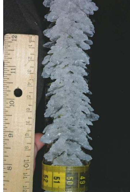
Figure 54. Complete scallops at \Lambda=45^\circ , V=200 mph, T=25^\circ\text{F} , \text{LWC}=0.75\text{g/m}^3 , \text{MVD}=20\mu\text{m} , \tau=5\text{min} . Direction of flow is from bottom to top, upper scale of ruler is in centimeters, smallest division 1 millimeter.
