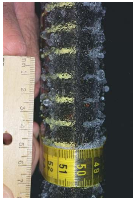
Figure 27. Front view of the ice accretion showing the attachment line zone and the glaze ice feathers zone. \Lambda=0^\circ , V=100 mph, T=25^\circ\text{F} , \text{LWC}=0.75\text{g/m}^3 , \text{MVD}=20\mu\text{m} , \tau=5\text{min} . Scale of ruler is in centimeters, smallest division 1 millimeter.
