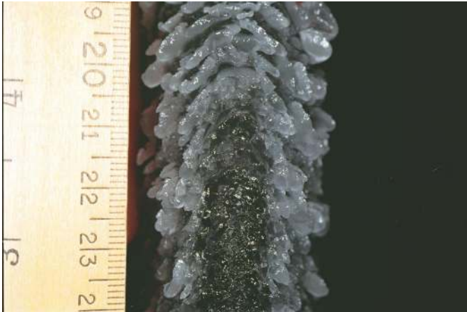
Figure 57. Front view of the beginning of the end cap showing the effect of the local sweep angle on the ice accretion. \Lambda=20^\circ , V=150 mph, T=25^\circ\text{F} , \text{LWC}=0.5\text{g}/\text{m}^3 , \text{MVD}=20\mu\text{m} , \tau=5\text{min} . Direction of flow is from bottom to top, scale of ruler is in centimeters, smallest division 1 millimeter.
