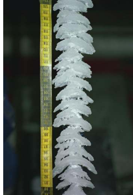
Figure 11. Front view of ice accretion. Run conducted with 1996 spray system. \Lambda=45^\circ , V=250 mph, T=25^\circ\text{F} , \text{LWC}=0.75\text{g/m}^3 , \text{MVD}=20\mu\text{m} , \tau=10\text{min} . Direction of flow is from bottom to top, scale of ruler is in centimeters, smallest division 1 millimeter.
