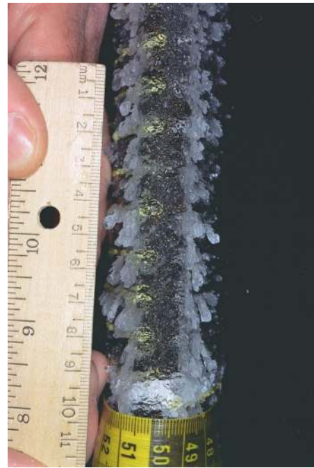
Figure 25. Front view of ice accretion showing the feathers forming scallop tips. \Lambda=30^\circ , V=75 mph, T=25^\circ\text{F} , \text{LWC}=0.8\text{g/m}^3 , \text{MVD}=20\mu\text{m} , \tau=10\text{min} . Direction of flow is from bottom to top, scale of ruler is in centimeters, smallest division 1 millimeter.
