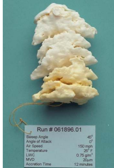
Figure 3. Urethane casting of an ice accretion.
