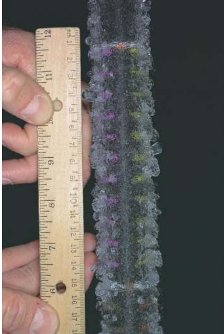
Figure 41. Front view of ice accretion showing the attachment line zone and the glaze ice feathers zone, with the feathers not forming scallop tips. \Lambda=10^\circ , V=150 mph, T=25^\circ\text{F} , \text{LWC}=0.75\text{g/m}^3 , \text{MVD}=20\mu\text{m} , \tau=5\text{min} . Direction of flow is from bottom to top, scale of ruler is in centimeters, smallest division 1 millimeter.
