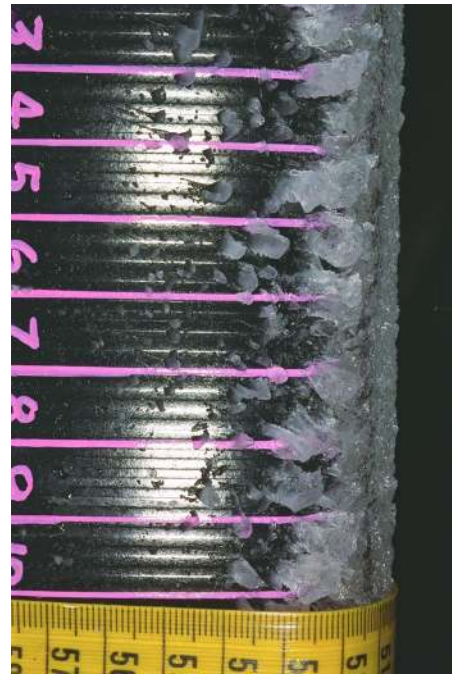
Figure 44. Side view of the ice accretion showing the feathers in the glaze ice feathers zone forming scallop tips. \Lambda=25^\circ , V=150 mph, T=25^\circ\text{F} , \text{LWC}=0.75\text{g/m}^3 , \text{MVD}=20\mu\text{m} , \tau=5\text{min} . Direction of flow is from bottom to top, upper scale of ruler is in centimeters, smallest division 1 millimeter.
