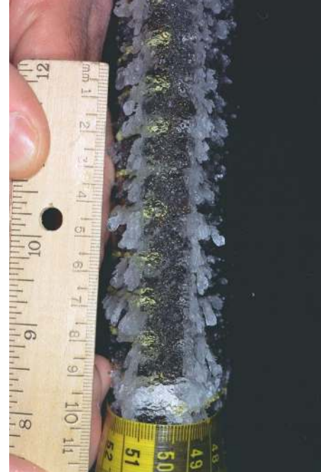
Figure 23. Front view of the ice accretion showing the orientation of the preferred direction of growth of the feathers. \Lambda=15^\circ , V=75 mph, T=25^\circ\text{F} , \text{LWC}=0.8\text{g/m}^3 , \text{MVD}=20\mu\text{m} , \tau=10\text{min} . Direction of flow is from bottom to top, scale of ruler is in centimeters, smallest division 1 millimeter.
