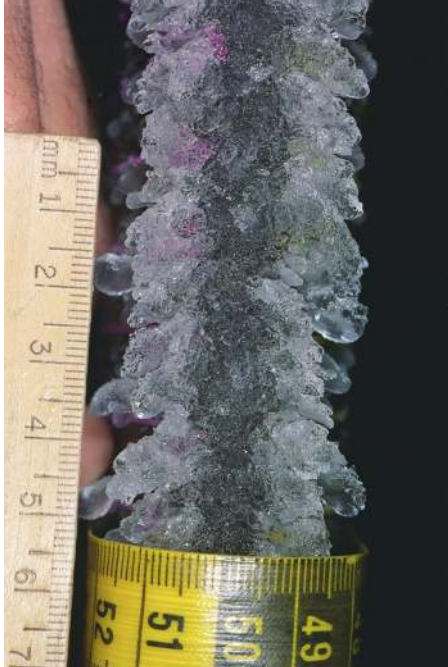
Figure 45. Front view of ice accretion showing scallop tips and the attachment line zone. \Lambda=35^\circ , V=150 mph, T=25^\circ\text{F} , \text{LWC}=0.75\text{g/m}^3 , \text{MVD}=20\mu\text{m} , \tau=5\text{min} . Direction of flow is from bottom to top, scale of ruler is in centimeters, smallest division 1 millimeter.
