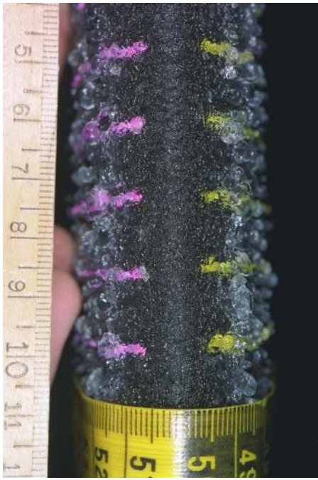
Figure 4. Front view of ice accretion at 2 minutes, showing the attachment line zone and the glaze ice feathers zone. Run conducted with 1998 spray system. \Lambda=15^\circ , V=150 mph, T=25^\circ\text{F} , \text{LWC}=0.75\text{g/m}^3 , \text{MVD}=20\mu\text{m} , \tau=2\text{min} . Direction of flow is from bottom to top, scale of ruler is in centimeters, smallest division 1 millimeter
