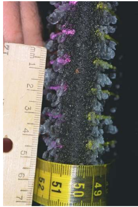
Figure 29. Front view of ice accretion showing the attachment line zone and the glaze ice feathers zone. \Lambda=25^\circ , V=100 mph, T=25^\circ\text{F} , \text{LWC}=0.75\text{g/m}^3 , \text{MVD}=20\mu\text{m} , \tau=5\text{min} . Direction of flow is from bottom to top, scale of ruler is in centimeters, smallest division 1 millimeter.
