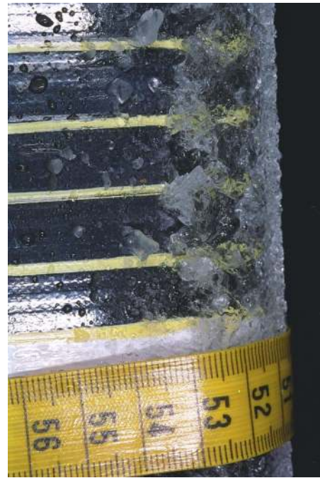
Figure 40. Side view of the ice accretion showing the ice of the attachment line zone covering the feathers in the glaze ice feathers zone. \Lambda=0^\circ , V=150 mph, T=25^\circ\text{F} , \text{LWC}=0.75\text{g/m}^3 , \text{MVD}=20\mu\text{m} , \tau=5\text{min} . Scale of ruler is in centimeters, smallest division 1 millimeter.
