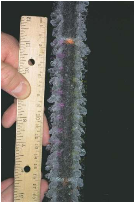
Figure 43. Front view of ice accretion showing the formation of scallop tips. \Lambda=25^\circ , V=150 mph, T=25^\circ\text{F} , \text{LWC}=0.75\text{g/m}^3 , \text{MVD}=20\mu\text{m} , \tau=5\text{min} . Direction of flow is from bottom to top, scale of ruler is in centimeters, smallest division 1 millimeter.
