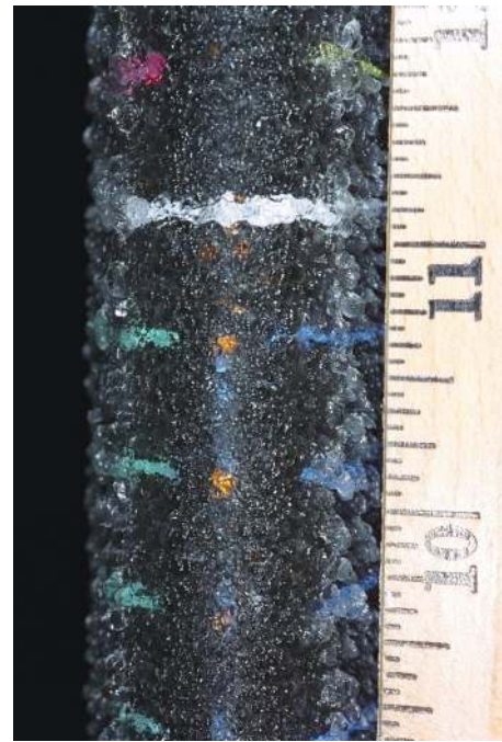
Figure 5. Front view of ice accretion at 2 minutes, showing the attachment line zone and the glaze ice feathers zone. Run conducted with 1996 spray system. \Lambda=15^\circ , V=150 mph, T=25^\circ\text{F} , \text{LWC}=0.75\text{g/m}^3 , \text{MVD}=20\mu\text{m} , \tau=2\text{min} . Direction of flow is from bottom to top, scale of ruler is in inches.
