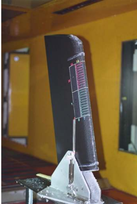
Figure 2. NACA 0012 swept wing tip in the IRT Test Section
