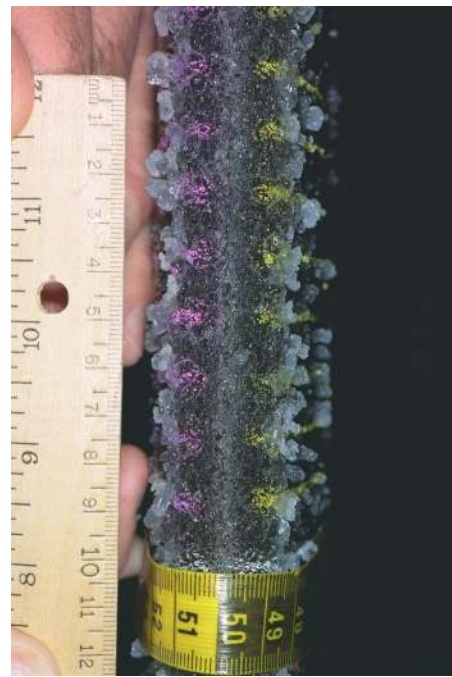
Figure 13. Front view of ice accretion, showing the attachment line zone and the glaze ice feathers zone at \Lambda=0^\circ , V=75 mph, T=25^\circ\text{F} , \text{LWC}=0.8\text{g/m}^3 , \text{MVD}=20\mu\text{m} , \tau=10\text{min} . Scale of ruler is in centimeters, smallest division 1 millimeter.
