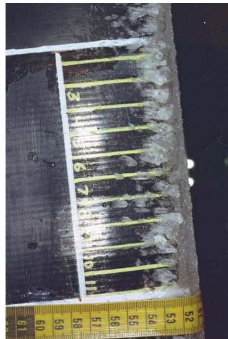
Figure 35. Side view of ice accretion showing the feathers in the glaze ice feathers zone. \Lambda=15^\circ , V=100 mph, T=25^\circ\text{F} , \text{LWC}=0.75\text{g}/\text{m}^3 , \text{MVD}=20\mu\text{m} , \tau=10\text{min} . Direction of flow is from bottom to top, scale of ruler is in centimeters, smallest division 1 millimeter.
