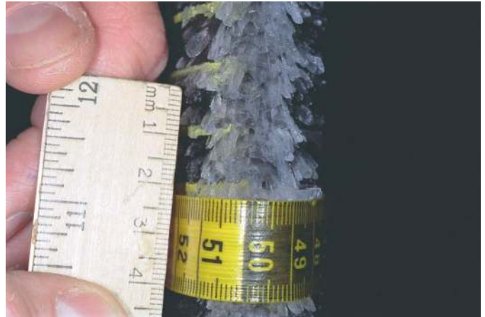
Figure 33. Complete scallop at \Lambda=45^\circ , V=100 mph, T=25^\circ\text{F} , \text{LWC}=0.75\text{g}/\text{m}^3 , \text{MVD}=20\mu\text{m} , \tau=5\text{min} . Direction of flow is from bottom to top, scale of ruler is in centimeters, smallest division 1 millimeter.
