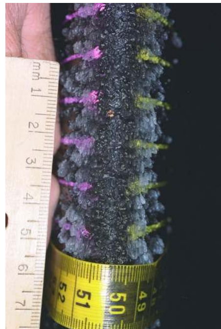
Figure 15. Front view of ice accretion showing the attachment line zone and the glaze ice feathers zone at \Lambda=30^\circ , V=75 mph, T=25^\circ\text{F} , \text{LWC}=0.8\text{g/m}^3 , \text{MVD}=20\mu\text{m} , \tau=5\text{min} . Direction of flow is from bottom to top, scale of ruler is in centimeters, smallest division 1 millimeter.
