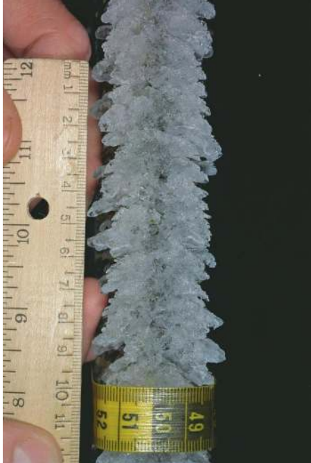
Figure 53. Front view of ice accretion showing complete scallops. \Lambda=40^\circ , V=200 mph, T=25^\circ\text{F} , \text{LWC}=0.75\text{g/m}^3 , \text{MVD}=20\mu\text{m} , \tau=5\text{min} . Direction of flow is from bottom to top, scale of ruler is in centimeters, smallest division 1 millimeter.
