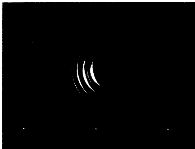
Fig. 2(b). The Fabry-Perot fringe system with 250-mW power input at 8.9 Gc. The new intermediate circles indicate the presence of an optical beam shifted by 8.9 Gc.
