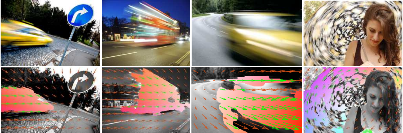
Figure 5. The blurry images (top row) show regions with significant motion blur, as well as static parts. Our algorithm estimates non-uniform motion for all blurry regions and segments out regions dominated by this blur (bottom row, color coding see text).
