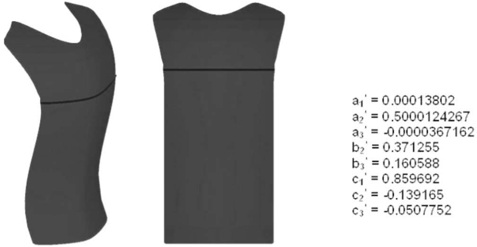
Fig. 8. Nominal isogeodesic surface with its parameters.
