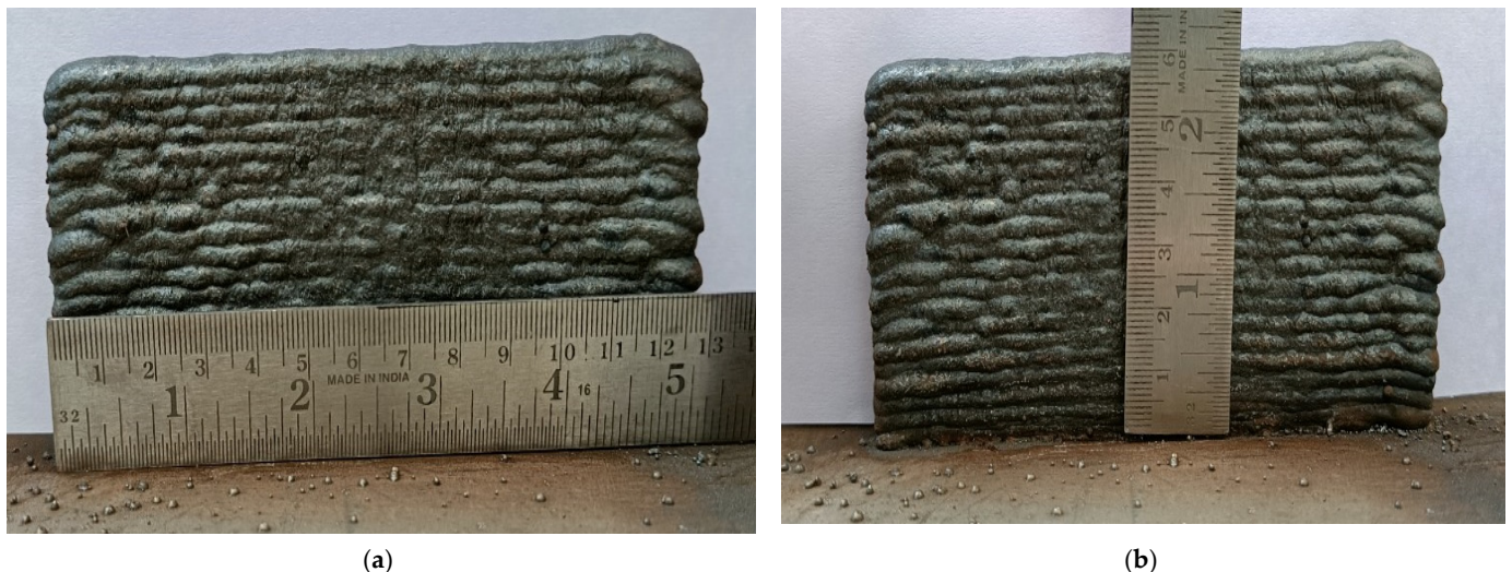
Figure 11. Multi-layered structure showing (a) length and (b) width on SS 316L substrate.
