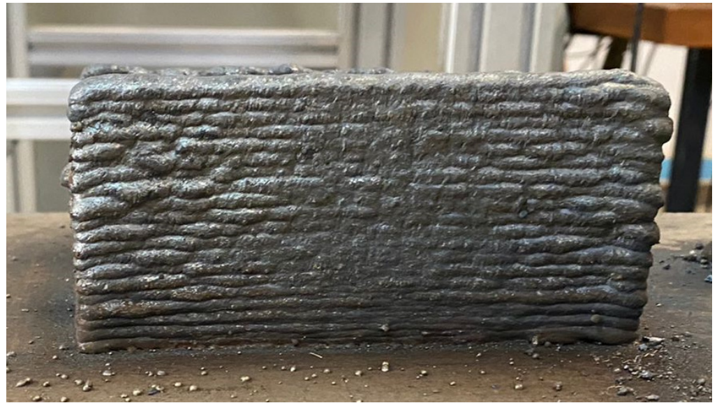
Figure 10. Multi-layered structure from WAAM process on SS 316L substrate.
