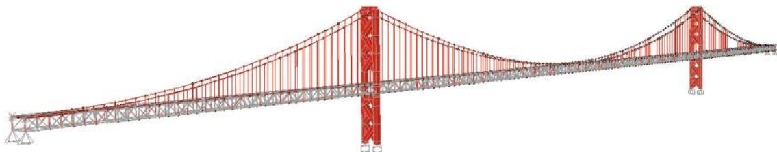
Fig. 17 Computer model of the Tagus bridge made in SAP2000
