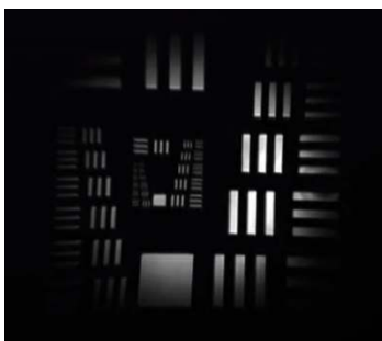
Fig. 33. Adapted from the supplementary material of [168]. Upconverted image of a USAF resolution target at 3.37 \mu\text{m} while rotating the crystal with respect to c-axis by 1^\circ and in synchronism with the camera integration time of 2.5 ms.
