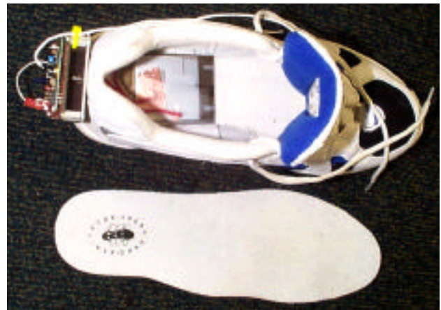
Figure 11: Sneaker-mounted tag circuitry and PZT element
