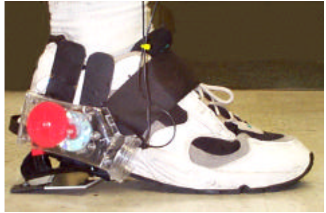
Figure 6: Simple shoe-mounted rotary magnetic generator
