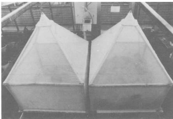
FIG. 2. Dispersal cages used to measure plant-leaving rate. Cages contained 1, 4, or 16 plants and 0, 10, or 100 aphids; eight wasps were released in each cage. Wasps that left patches flew upward and were trapped in vials.
