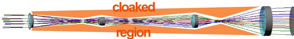
FIG. 3. CODE V simulation of a symmetric, perfect paraxial cloak, with four lenses using rays. Four achromatic doublets are placed with separations determined from equation (5). Entrance pupil is 50 mm, with -1.5^\circ to 1.5^\circ field-of-view. Simulations are shown with no separate optimization. Object is placed at infinity.
