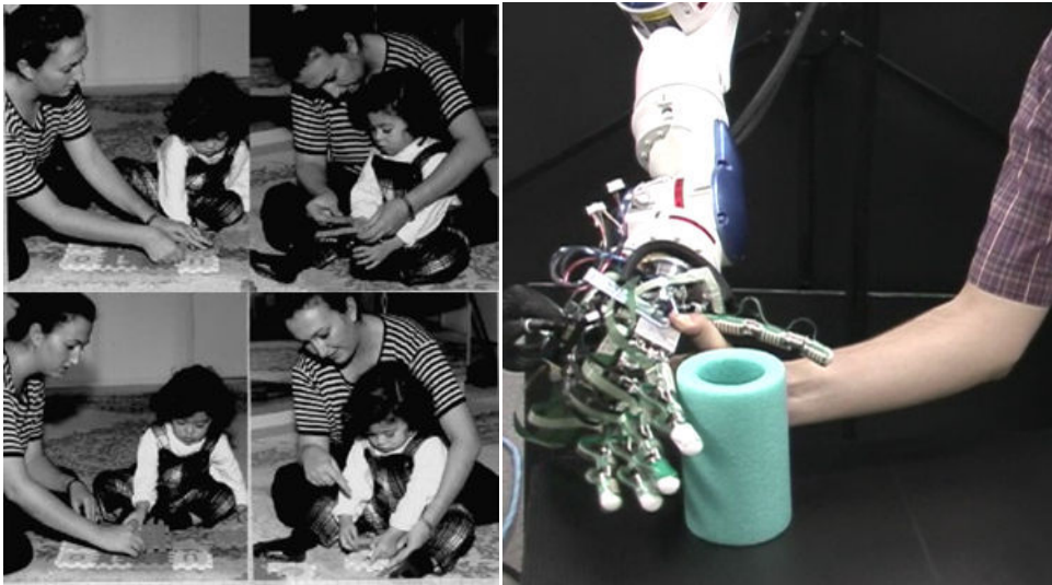
Fig. 1. Left: The caregivers step in when the task of the child gets out of hand. They teach infants different skills by highlighting important features of the task or marking the boundaries of action units. Right: 7 DoF robot arm, 16 DoF robot hand, table, and a sample object is shown. The range camera is placed on the top-right and not visible. The human teacher can change the default trajectory of the robot to enable grasping thanks to the force/torque sensor that is placed between robot arm and hand.
