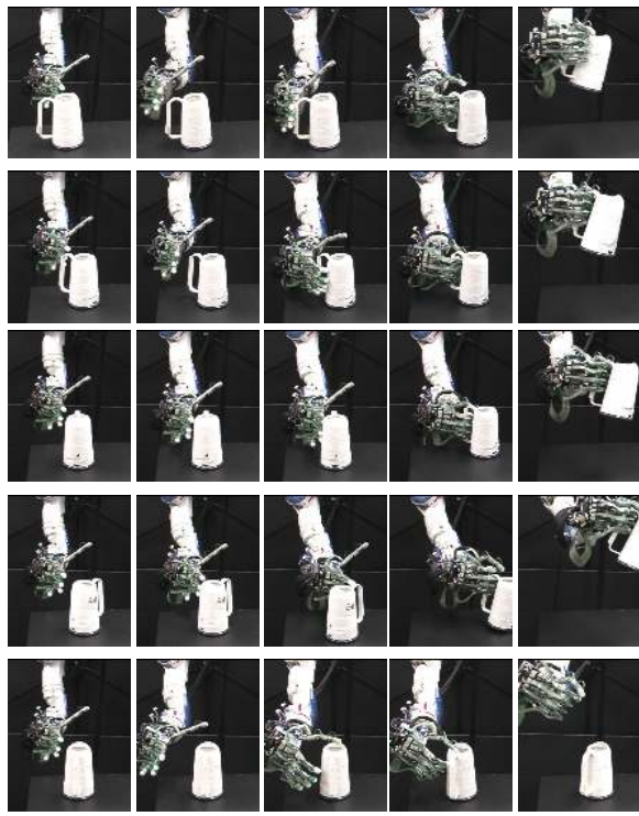
Fig. 6. Robot grasps objects using the trajectories learned during scaffolding. Each row corresponds to a different grasp execution.
