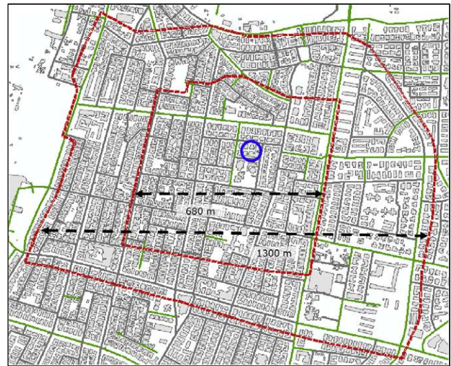
Fig. 6. The two concentric rings employed for estimating the effects of a new parking lot in the Basel neighborhood.
