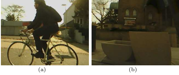
Figure 12: (a) A moving bicyclist, and (b) a flowerpot, both objects that produced dips in the sensor trace that were classified incorrectly as parked cars
