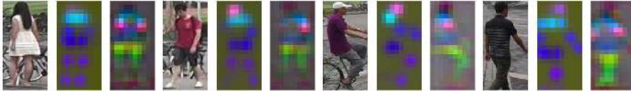
Fig. 5. Comparing the body part descriptors. For a given image (left), the conventional joint-based (center) and the proposed (right) descriptors are visualized. (Best viewed in color)
