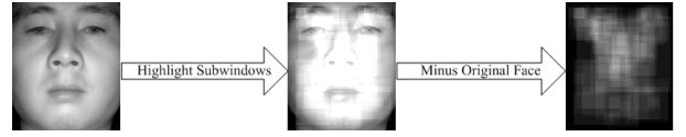
Figure 2. The first 100 subwindows of SLBPH feature learned by AdaBoost. Only the highlighted facial parts are contributed in face recognition, and the brightest parts indicate the most discriminative power.
