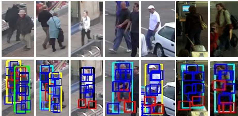
Figure 7. Examples results of our dynamic occlusion handling approach. Top row shows the original image, and bottom row shows the detected humans are their corresponding parts, where the occluded parts shown in red.
