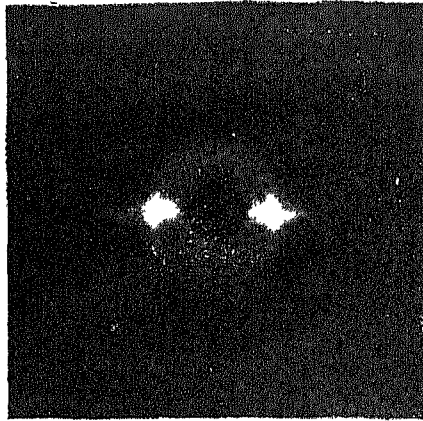
7 X-ray diagram of Tectona Grandis after heating
