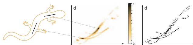
Figure 9: Reflective symmetries of a 2D lizard. Approximate reflective symmetry across the spline gets mapped to a curve in the 2D transformation space.
