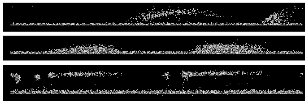
Figure 1. Examples of positive PRPD samples. Top: Internal discharge, Middle: Internal discharge from 22 kV bushing of oil-filed transformer, Bottom: Internal discharge from voids of solid insulator.
