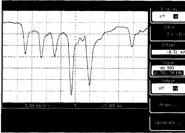
Figure 3.9 Superposition of consecutive discharges for voids with a large D/h ratio, D=20 mm, h=1 mm.
