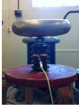
Figure 5.3: Test setup for surface discharge in air
