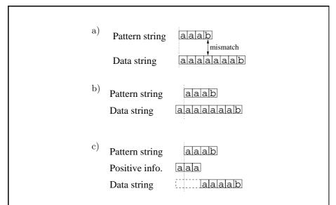
Figure 3: The role of positive information. a) A mismatch occurs. To the left of the mismatch, pattern string and data string are equal (positive information). b) Restart of the straightforward matcher. The pattern string is shifted one position to the right and matching resumes by comparing the pattern string with the data string. c) Restart of a matcher that specializes well. Positive information has been collected, and matching resumes by comparing the pattern string against it.
