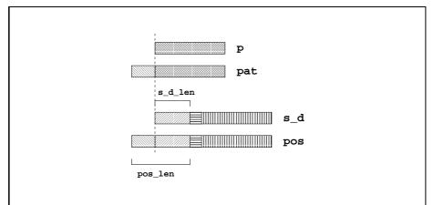
Figure 22: Interdependencies between the arguments of match\_s as proven by Lemma 18. Parts of the strings that have the same shading are equal.
