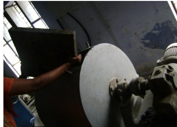
Fig. 1: crushing of glass pieces using loss angles machine
