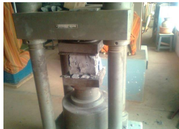
Fig. 3: UTM for compressive strength
