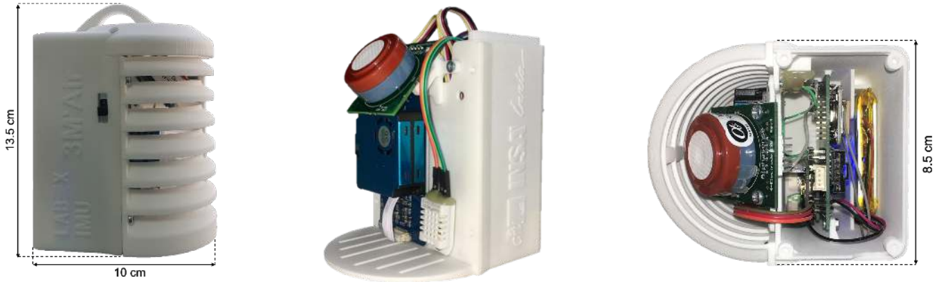
Fig. 2. (a) External side view of the designed sensor node; (b) Internal side view (sensor chamber); (c) Internal top view (second and third chambers)
