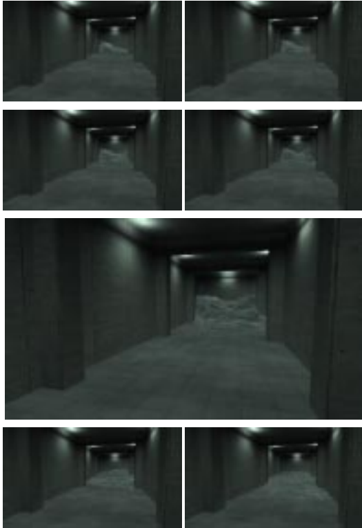
Figure 2: Corridor flood simulation. The fluid motion is simulated by 100,000 fluid particles. The simulation time is about 3 minutes per frame.
