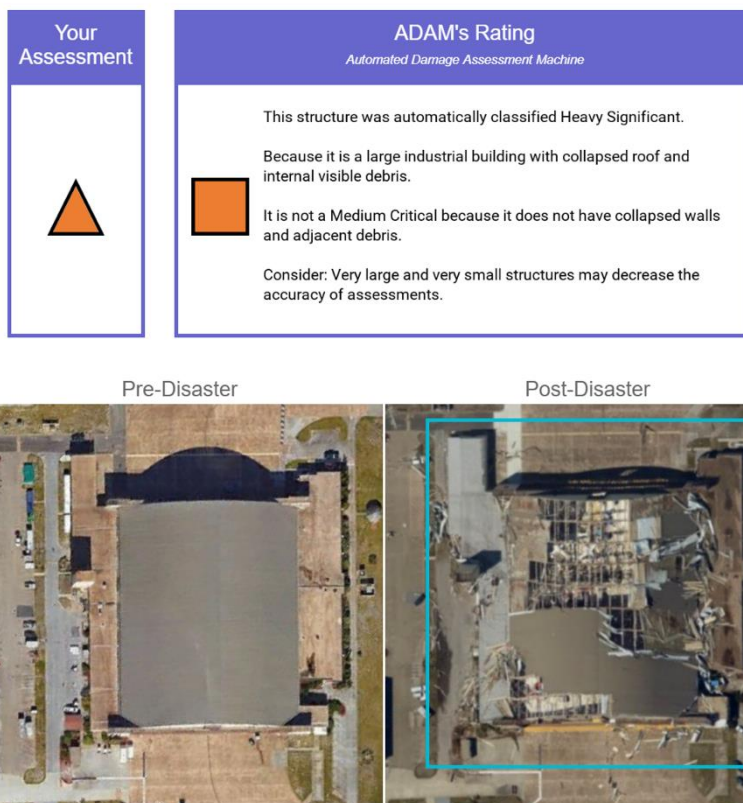
Figure 2 Example Damage Classification and Explanation
