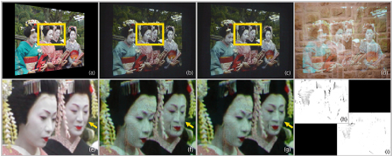
Figure 5: Passive calibration results: ideal image (a) and close-up (e), uncorrected image (b) and close-up (f), corrected image (c) and close-up (g), image without radiometric compensation under environment light (d), visualized error maps for uncorrected (h) and corrected (i) case.
