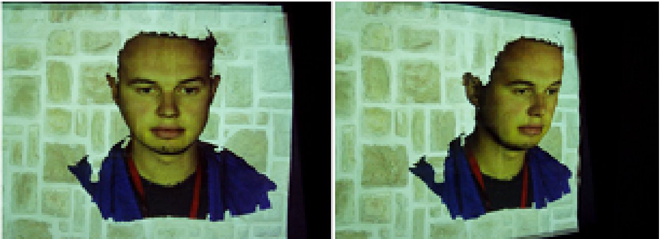
Figure 1: View-dependent stereoscopic projection of 3D content onto large natural stonewall.
