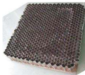
Figure 7. Honeycomb panel sample filled with paraffin, before to stick the upper aluminum skin [87].
