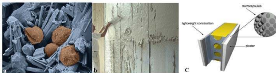
Figure 4. (a) Electron microscopy of PCM in gypsum plaster Micronal® [78]; (b) PCM gypsum plaster finishing on the wall ©BASF [79,80]; (c) PCM micro-capsules integrated into the interior plaster [61].
