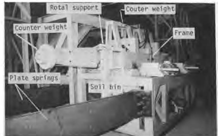
Fig. 1 Soil bin supported by plate springs
