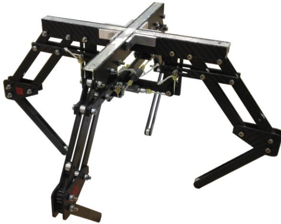
Figure 15 – Second prototype manufactured out of carbon fibre with a total weight of 378g suitable for small scale UAV use.
