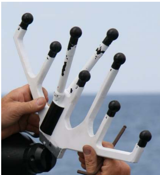
FIG. 4. (Color online) The passive acoustic array consisting of tetrahedral and line sub arrays. This was mounted to the nose of the eFolaga AUV.
