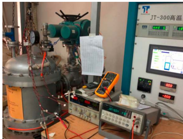
Figure 7. High-temperature and pressure calibration device developed by the authors.
