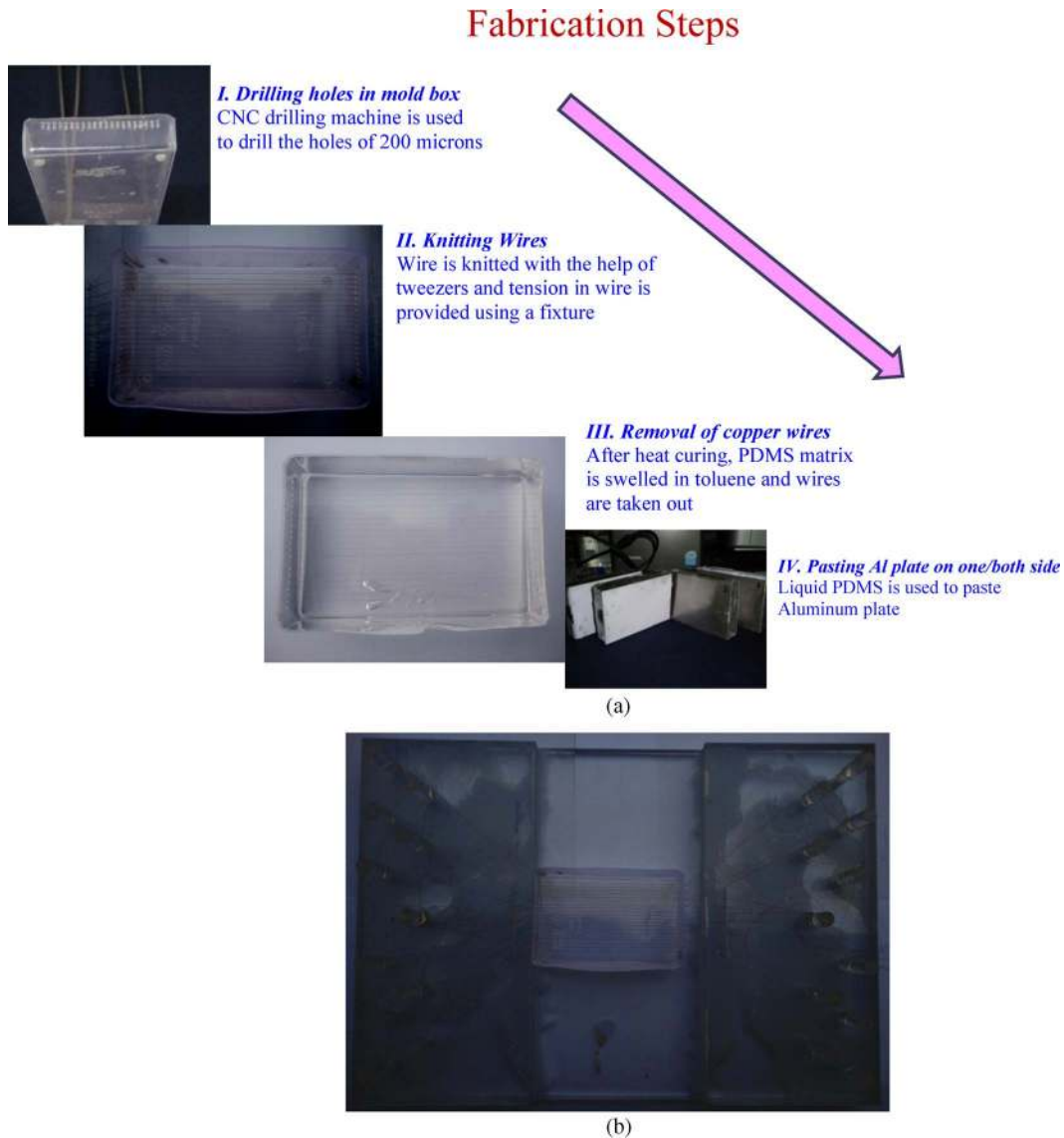
Fig. 2. (a) Different steps of fabrication of the damper assembly. (I) Drilling holes in the plastic mold. (II) Inserting the wire array and using the fixture to provide longitudinal tension for consistency of the microchannels and replication with PDMS. (III) Removal of the molding wires to obtain a straight array of microchannels. (IV) Pasting the aluminum plates at the bottom for unconstrained damping and at both top and bottom for constrained damping. (b) Tensioner fixture for tightening the replicating wires to ensure straightness of the features.
