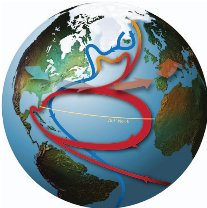
FIG. 1. A simplified schematic of the AMOC showing both the overturning and gyre recirculation components. Warm water flows north in the upper ocean (red), gives up heat to the atmosphere (atmospheric flow gaining heat represented by the changing color of broad arrows), sinks, and returns as a deep cold flow (blue). Latitude of the 26.5°N AMOC observations is indicated. Note that the actual flow is more complex. For example, see Bower et al. (2009, their Fig. 1) for the intermediate depth circulation in the vicinity of the Grand Banks and Biastoch et al. (2008, their Fig. 2) for the middepth circulation around South Africa, showing the importance of eddies in transferring heat and salt from the Indian Ocean to the Atlantic Ocean.
