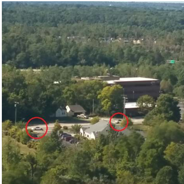
Figure 6. Artificial movers are injected into the median-filtered background image and are circled in red.
