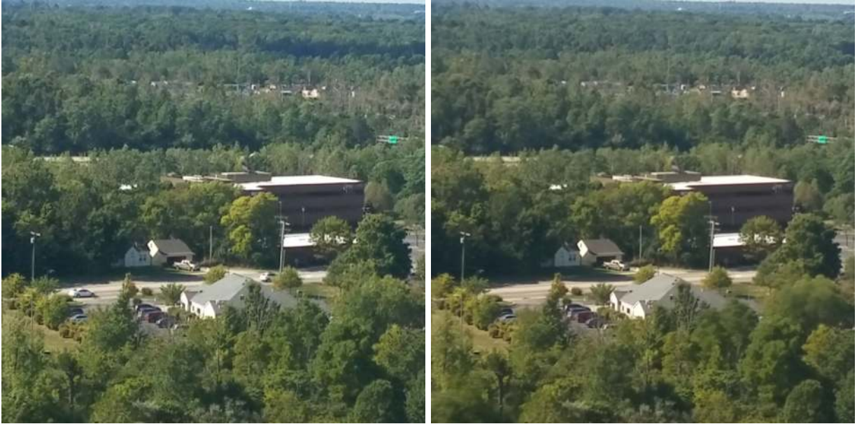
Figure 5. The left image is a typical raw image from a video, and the right image is the result of applying a median filter to the 600-frame image registered temporal median. Note the white car on the left is eliminated on the right due to its motion.
