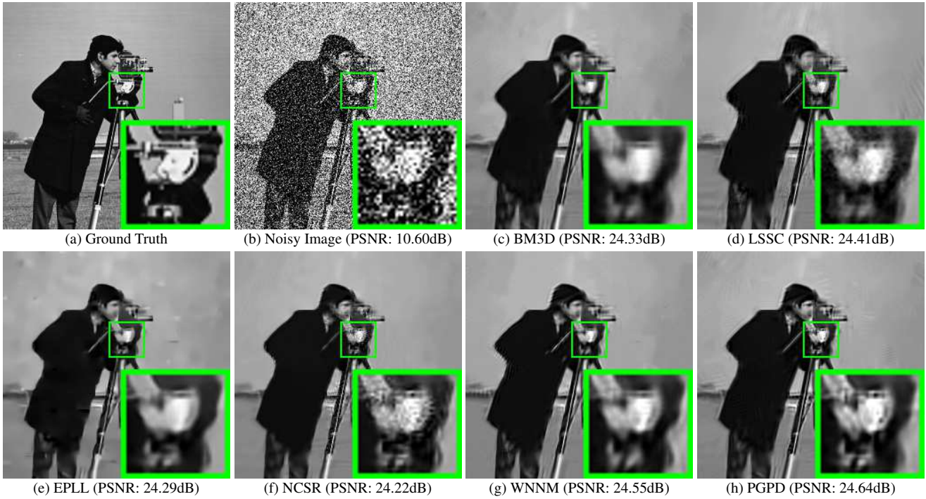
Figure 7. Denoised images of Cameraman by different methods (the standard deviation of noise is \sigma = 75 ).
